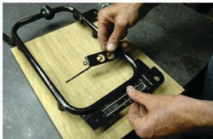
Install new spring clip
