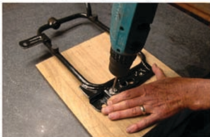
Drill out the two aluminum rivits
