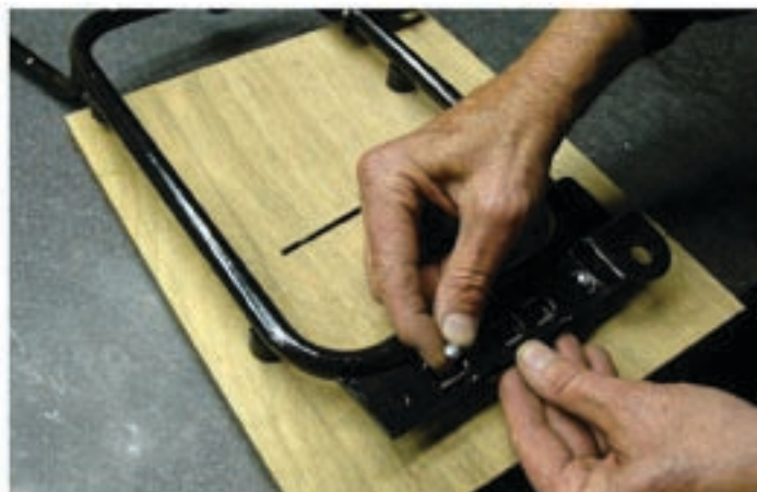
Replace rivits with the provided 10-32 screws and lock nuts
